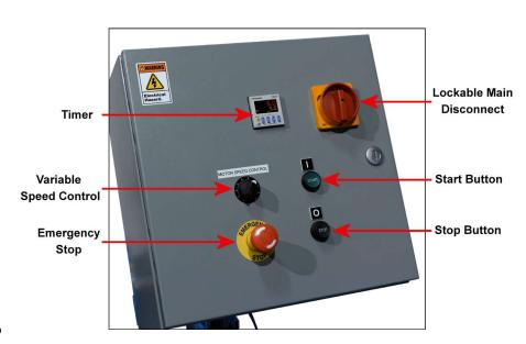
Use variable speed knob to control drum rotation from 2 to 20 rpm.
